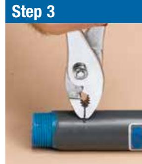
In **Step 3**, the tab is pulled perpendicular to the conduit with a pair of pliers. The plastic tab will tear off rather than having any peeling effect, or coating separating from the substrate.
